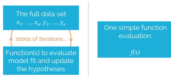
Figure 1: The difference between AI training (left) and AI inference (right): training needs all the data, and many iterations to determine model fit and adjust hypotheses. Inference needs a single example and only the selected hypothesis.
